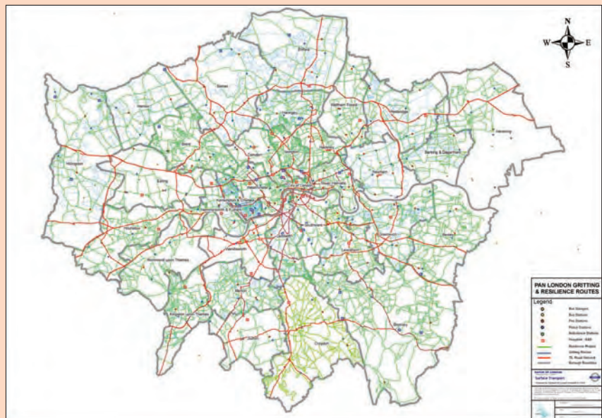
Figure T-09: The London Road Resilience Network. (London Councils, Crown Copyright, 2010)
