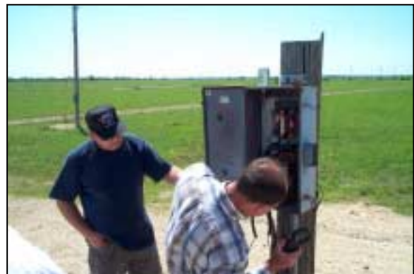
The split-ring current transformers (CTs) and voltage leads are installed at the pump jack electrical panel. Sensor leads are connected to the Amprobe and the unit is field configured.
