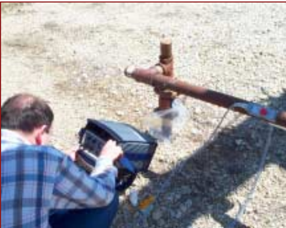
The flow meter is easily configured in the field. Key settings are pipe i.d., time interval, and units. Note the sensor on the pipe. For 24 hour logging the unit is placed in a weatherproof vented box.
