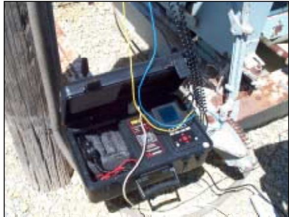
The Amprobe unit logging data. For 24 hour operation the unit is placed in a weatherproof plastic container with a small fan and vent.
