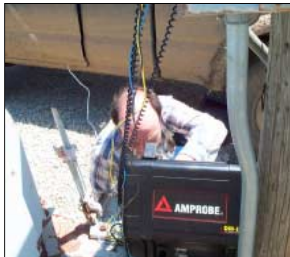
The split-ring current transformers (CTs) and voltage leads are installed at the pump jack electrical panel. Sensor leads are connected to the Amprobe and the unit is field configured.
