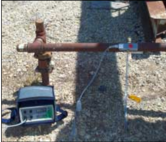
The Greyline portable Doppler flow meter in operation, providing accurate well fluid flow measurement without drilling or cutting the pipe.
