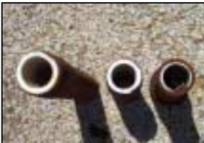
Accurate inside pipe diameter is required to acquire accurate flow data. Plastic lined pipe resists salt corrosion.
