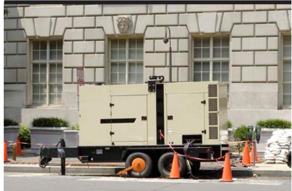
*Recommendation:* Electric utilities should increase the use of mobile generators to provide temporary power during a VLSE. During emergency planning processes, and well in advance of VLSEs, utilities should establish locations where generators can be easily connected and integrated into the grid. Similarly, they should upgrade and enhance control and monitoring systems to increase situational awareness and support the safe and reliable dispatch of DERs during VLSEs.
