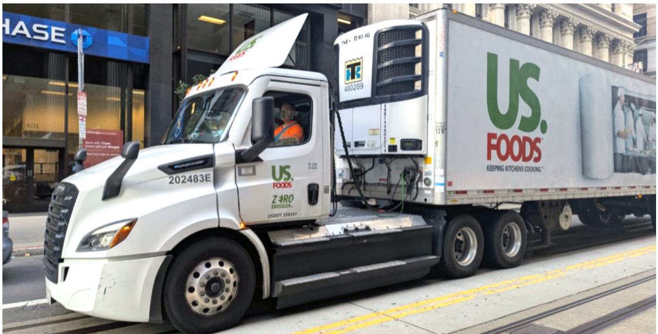
Figure 22: Class 8 Truck with TRU on the Trailer (Forum Mobility)
