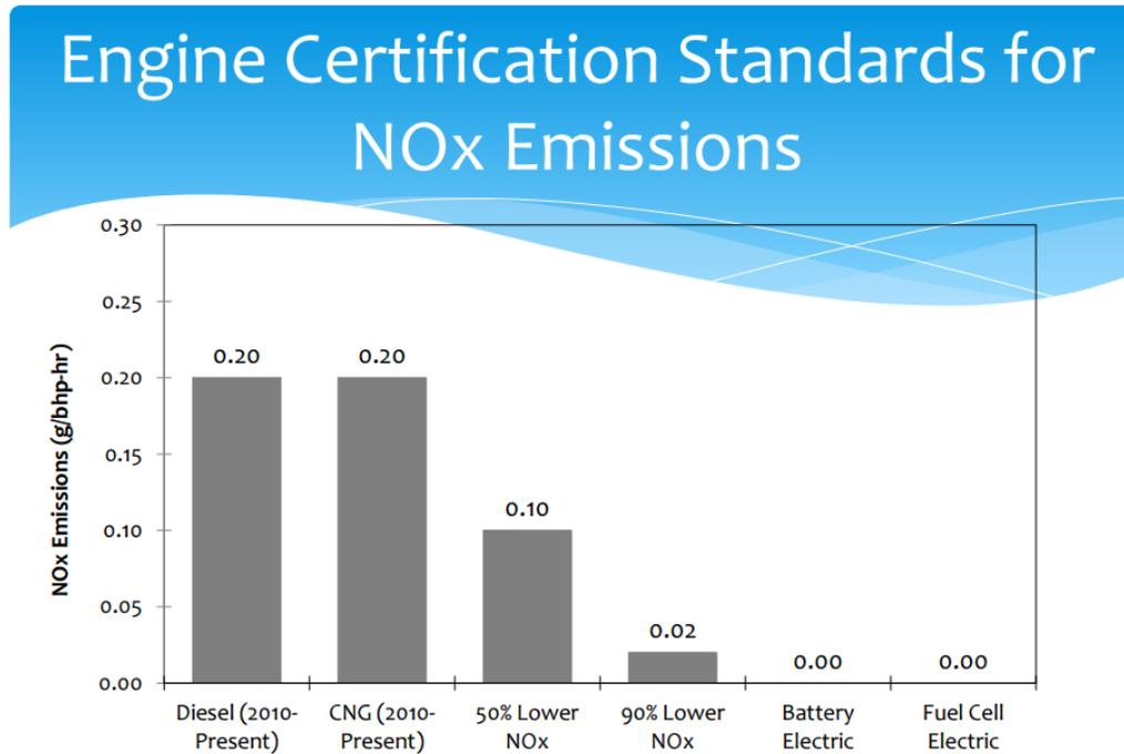
Figure 4 - CARB Engine Certification Standards for NOx Emissions<sup>11</sup>
