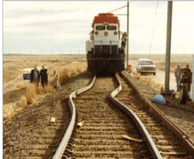
Track buckling is typically caused by a combination of high compressive forces due to temperature stresses, weakened track conditions, and mechanical stress from train braking and rolling friction. Safety and operations are therefore impacted by both extreme high and low temperatures, by causing track creep, and by making track more susceptible to the mechanical stresses that cause buckling.
