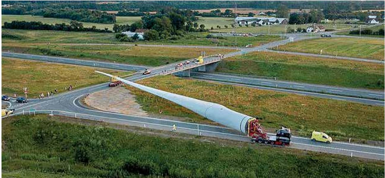
As wind turbines continue to grow in size, project developers will face greater challenges in transporting components. This 80-meter blade is being transported to a 7-MW test turbine in Scotland.
