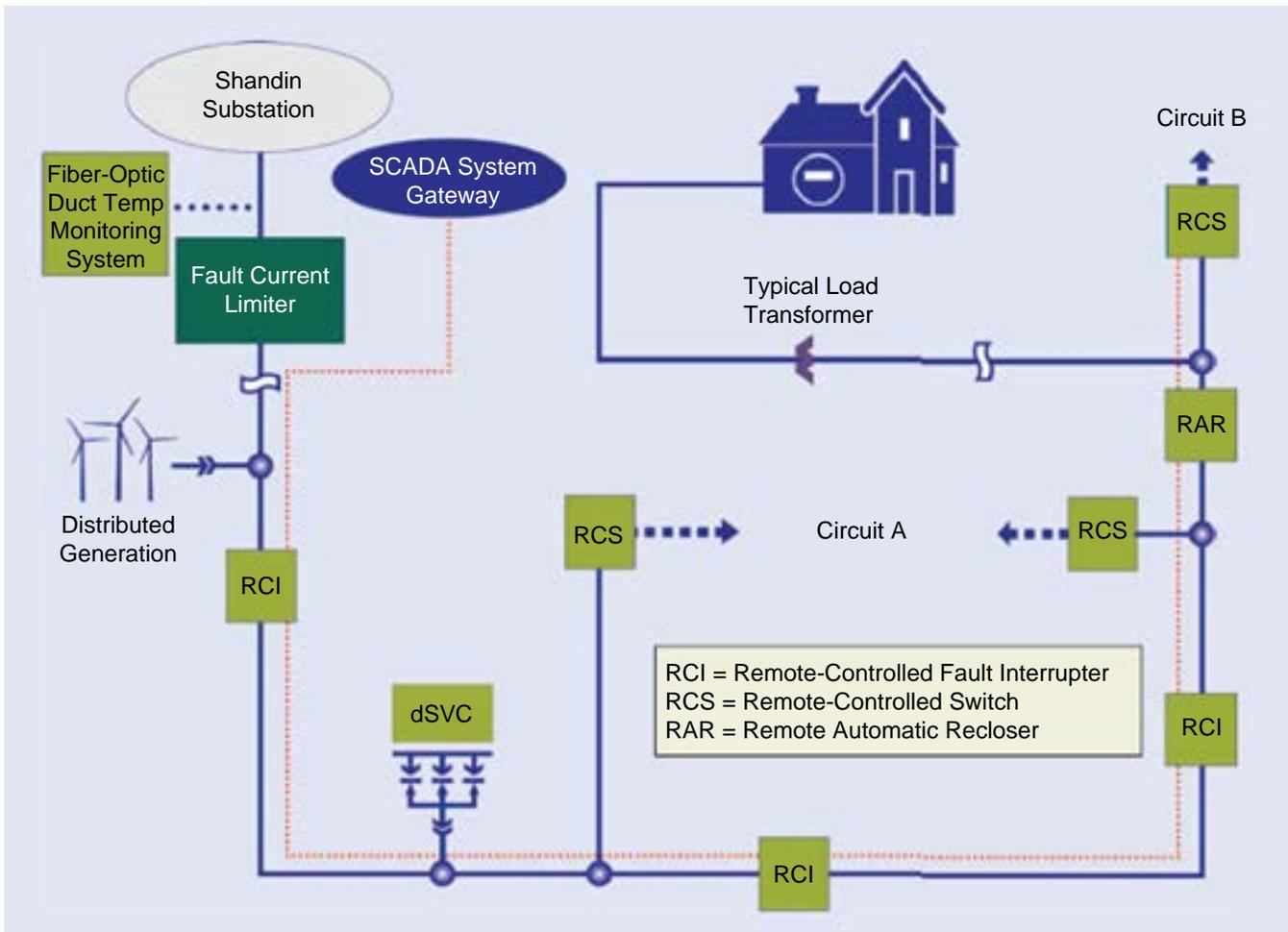
Figure 16. Circuit Auto-Reconfiguration (Graphic courtesy of Southern California Edison)
