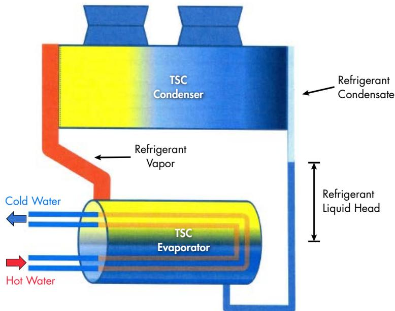
Figure 5. Flow Diagram for the TSC
